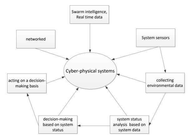
The main components and characteristics of cyber-physical systems
