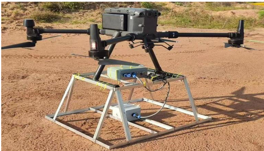
Figure 2. DSF Geopolariton tomography equipment based on the UAV
